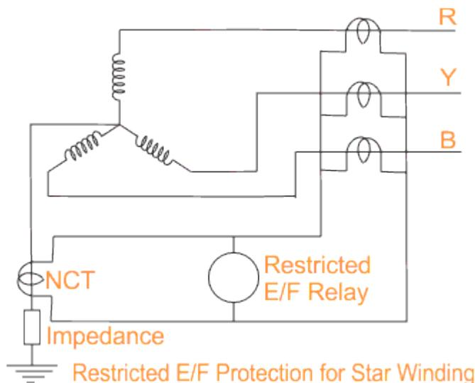
**Figure 5 - Restricted earth fault relay protection schematic**
