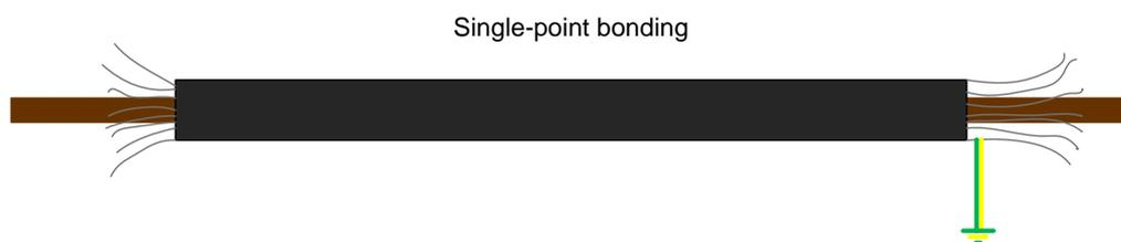
**Figure 2 - Single-point bonding of single core armoured cable**
