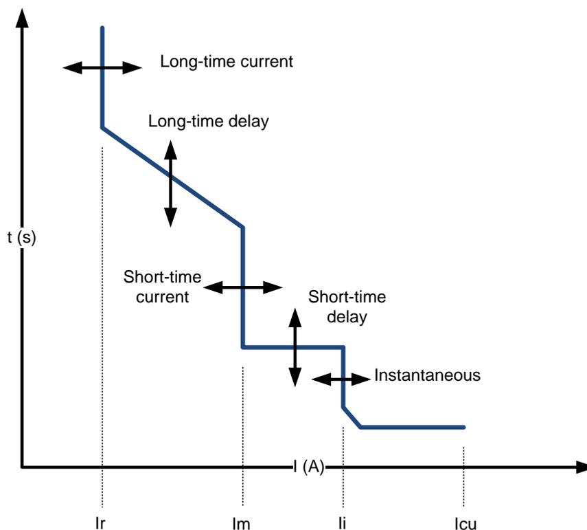
**Figure 4 - Tripping current ranges of low voltage MCCBs**
