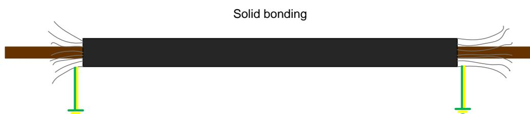
**Figure 3 - Solid bonding of single core armoured cable**
