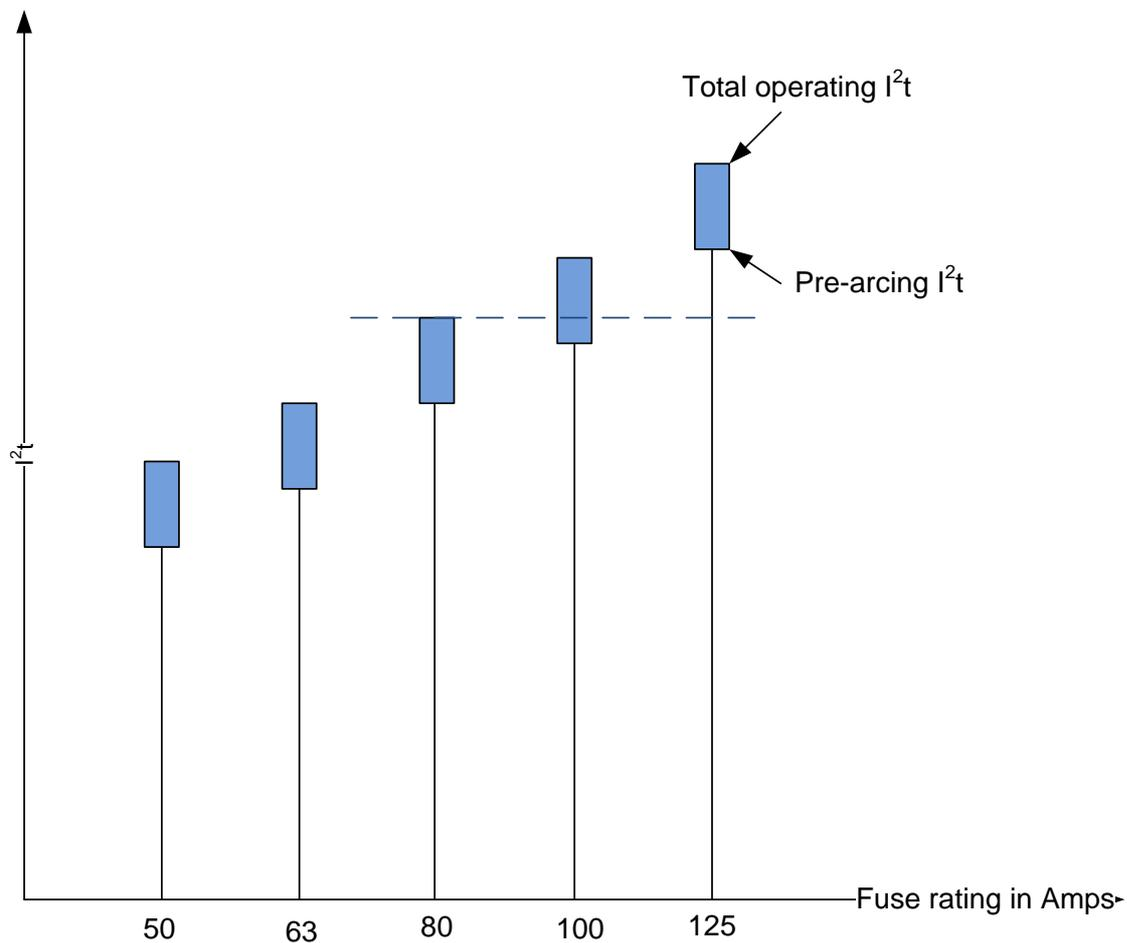
**Figure 7 - Example pre-arcing and total operating I<sup>2</sup>t values of fuses**
