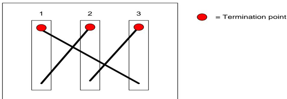
Figure 4 - Typical HV / LV terminations on a cast resin transformer
