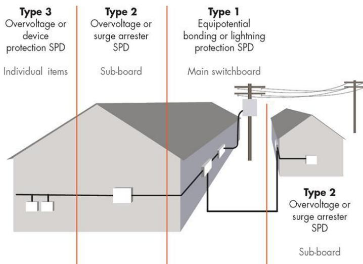
**Figure 10 - Typical layout of SPDs (taken from the IET on site guide)**
