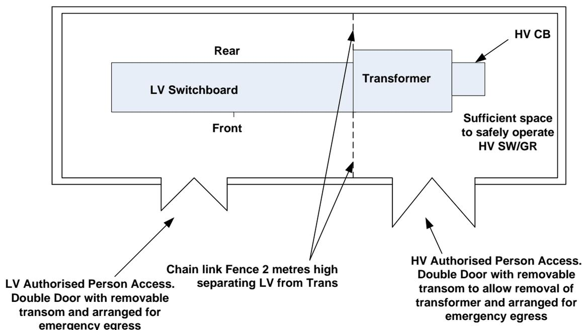
Figure 15 – Typical Layout of Packaged Substation 'Switch room'
